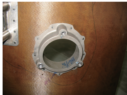
图3 安装在复合材料构件上的锁键螺套 Fig.3 Key-locking insert in the composites component
